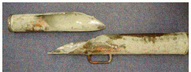
Photograph 2: Failed reducer—exploded view
